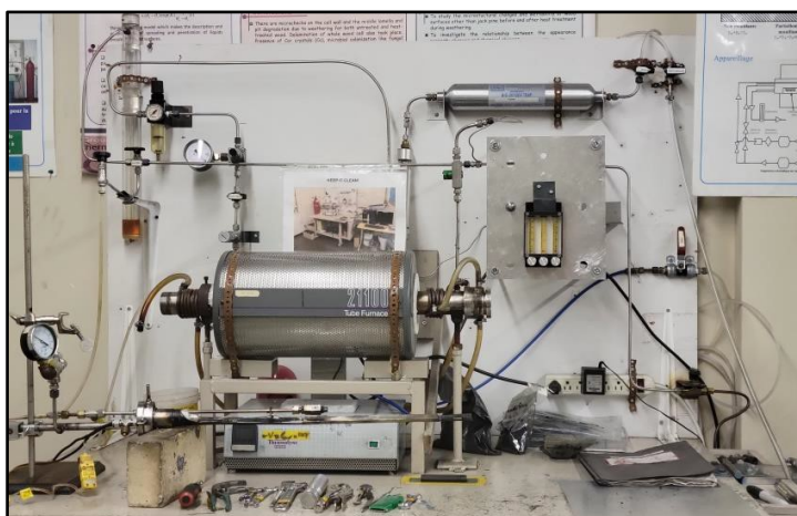
Figure 2. Sessile-drop system for wettability measurements at UQAC.
